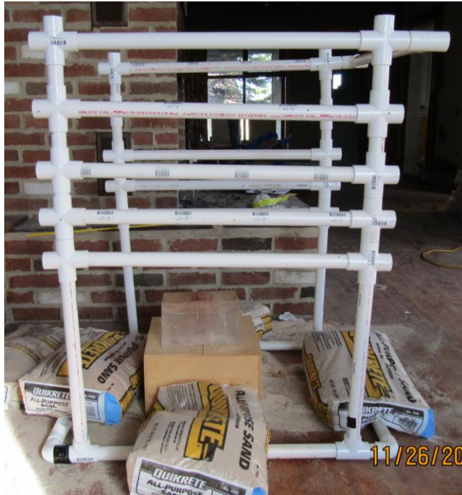
Figure 143. Device showing relationship between the ballistic gel target and slots for poster board.
