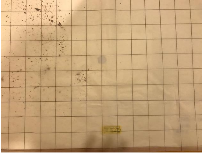
Figure 146. Grid placed over simulation in Figure 145 to quantify number of grids with blood spatter present.
